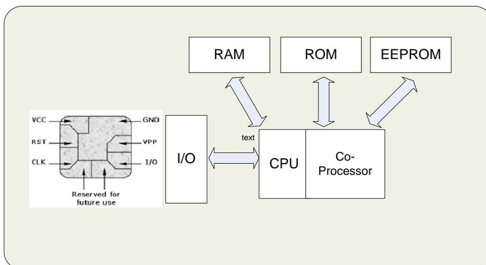
Figure 10: Smartcard components (without antenna) [45] [46]
