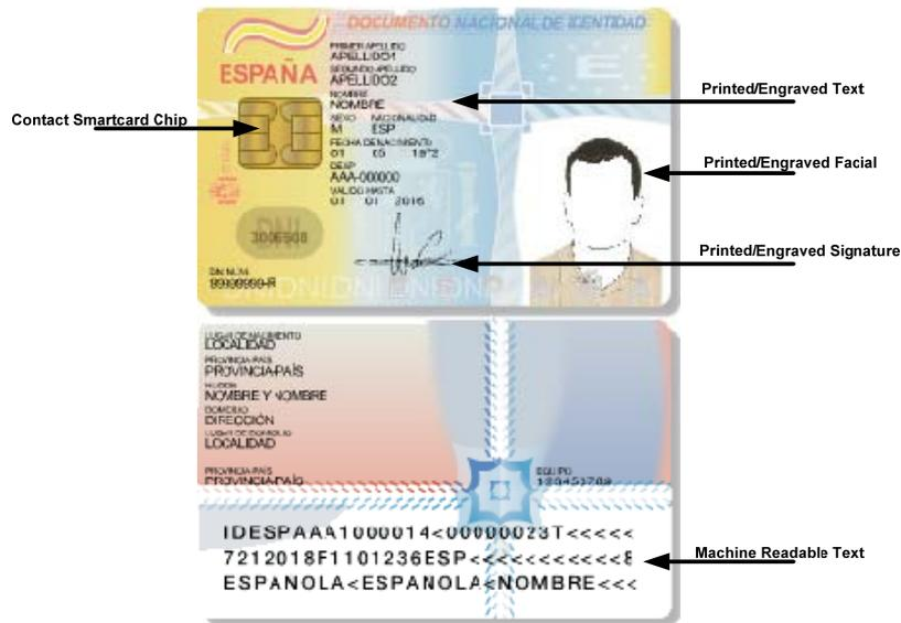
Figure 9: Some Key Components of an e-ID Card [41]
