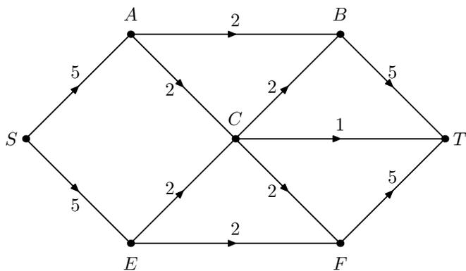
Find with proof a maximal flow in this network. What is its value?
